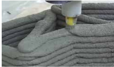
Top down multi-pass extrusion out of a generally round nozzle *2
