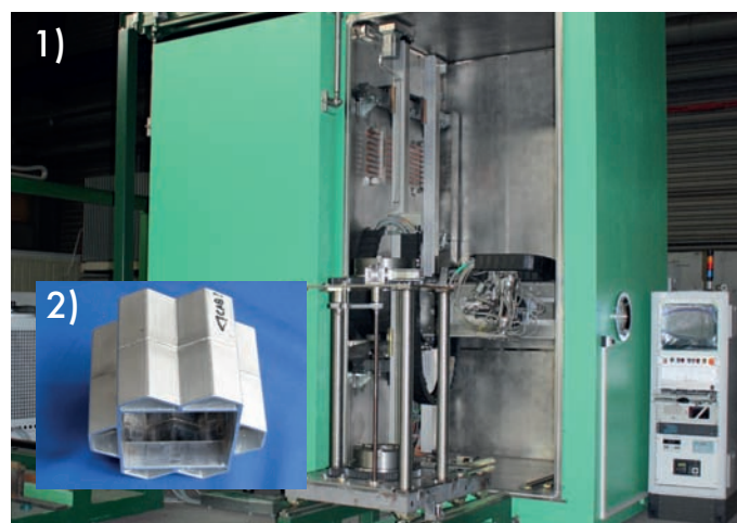
Fig. 1. Installation for the electron-beam welding. Fig. 2. Neutron-generating target body element.
