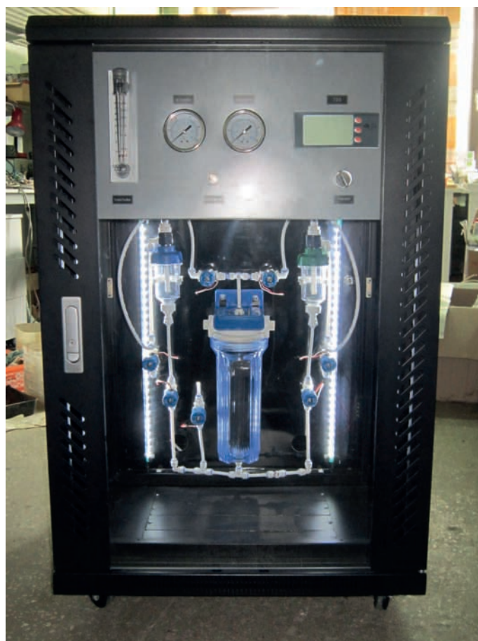
A working prototype of the electrolyzer developed during the project
